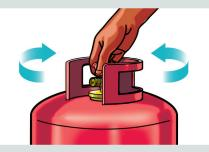
2 Check the valve functions properly and then close it before removing the safety seal.
