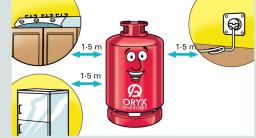
Always leave at least 1.5 metres between the cylinder and any source of heat, flame or sparks.
