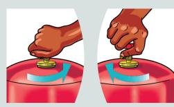
A half-turn of the valve is enough to open the cylinder and remember to close it after use.
